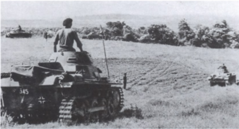
A Panzer regiment on field exercises, summer 1939. In the foreground is a Panzer I light tank, ahead of it a light Panzer II armed with a 20mm gun. To the left, in the background, are a Panzer III and Panzer IV medium tank, the first armed with a 37mm gun and the latter with a short-barrelled 75mm. (Private collection)
